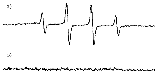
Figure 6. EPR spectra (DMPO as spin trap) obtained from aqueous suspensions of a) crocidolite, which shows the signal of the [HO \cdot -DMPO] adduct, and of b) crocidolite pretreated with F. oxysporum .
