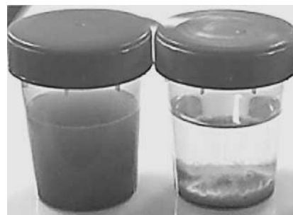
Figure 1. Effects of fungal mycelium on a suspension of asbestos. Fine asbestos fibers ( 1.5\text{--}4 \mu\text{m} mean diameter) form a turbid suspension when dispersed in the Czapek glucose medium (left). When the fungal mycelium, here the sterile mycelium strain MUT840, was grown in the medium containing asbestos fibers, it removed the fibers from the suspension, thus leaving a clear supernatant (right). This phenomenon was observed for all the fungi tested and indicates that the fungal hyphae can bind or entrap the asbestos material.
